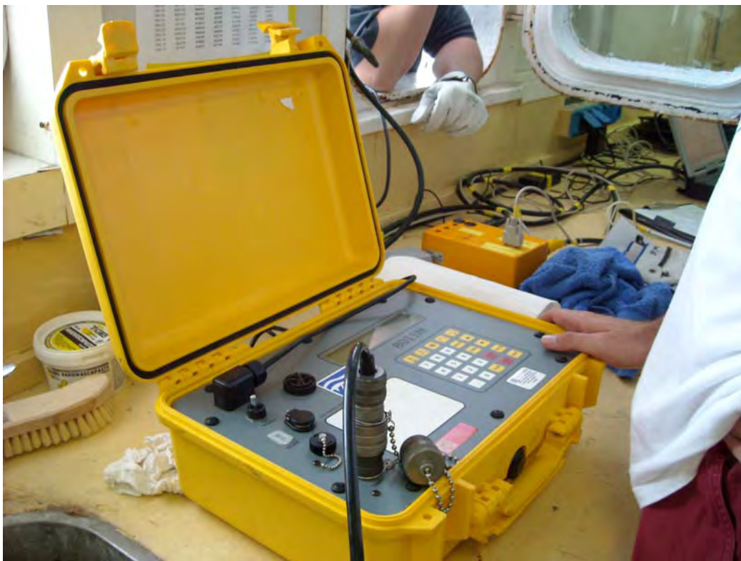
Figure 4. Deck unit 8011M used to communicate with the release unit of the OBS.
