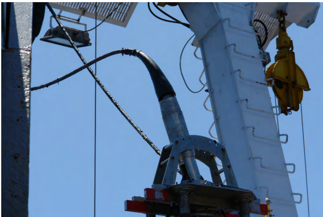
Fig. 38 - Termination and the bending restrictor before the Nearest recovery in August 2008
