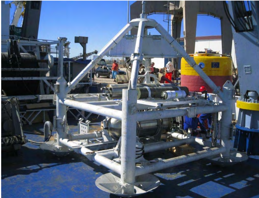
Fig. 31 - GEOSTAR abyssal multiparameter station
