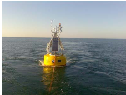
Figure 13 - The communication buoy just after the re-deployment in November 2009 when the second mission started.
