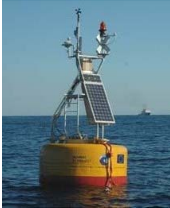
Figure 10 - The GEOSTAR pre-exposed buoy which hosts the surface devices of the Tsunameter.
