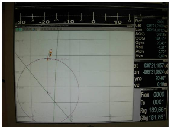
Figure 17 The navigation system locating the vessel during the GEOSTAR deployment procedures. The magenta circle represents the 200 m safety area from the dead weigh position
