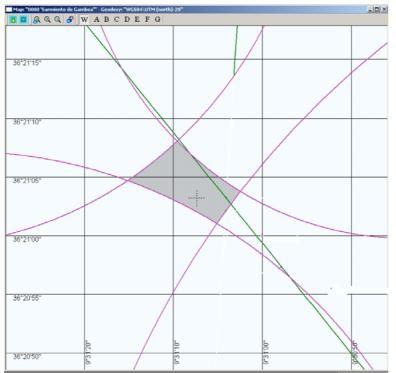
Figure 24 Preliminary graphical buoy DW localization. The magenta arcs of circle are centred in each of the four WPs of Tab. 1, their intersection gives the DW localization. The shaded region extend aprox. 250 times 120 meters is the candidate localization area after preliminary evaluation; the diagonal green line is the trip of the vessel during the deployment buoy operation (screen capture from the navigation system);
