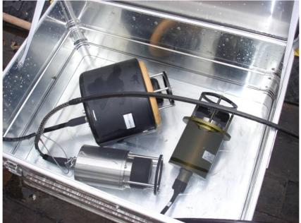
Figure 11 Acoustic transducer wet test
