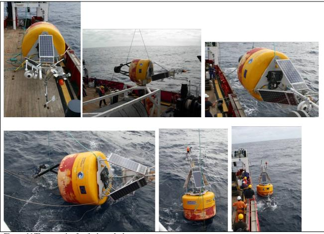
Figure 16 The operation for the buoy deployment
