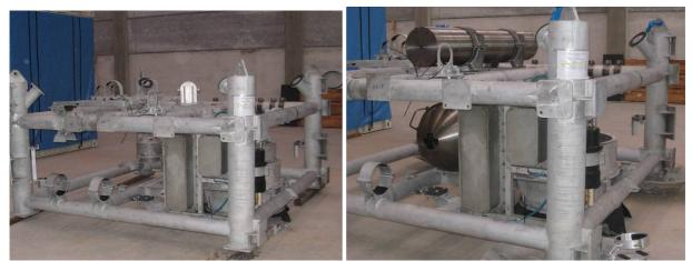
Figure 3 The beginning of the GEOSTAR assembling: the bare frame (left) and with the DACS, the battery vessel and assembled (right) .
