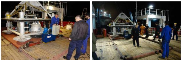
Figure 14 Commissioning of moving platform to support the deck operation
