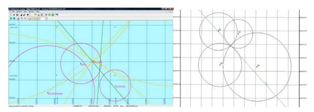
Figure 25 Geometric determination of dead weight position using 4 point of range measurements. The diagonal green line represent the route followed by the vessel during buoy deploymen; The yellow circles are centered each one in the four point of measure; B1-B5 are the points for acoustic localization, the circle intersections localizes the DW position.
