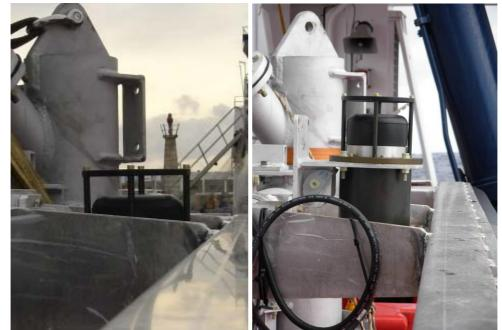
Figure 12 The acoustic transducer installed on GEOSTAR: original position (left), new position (right)
