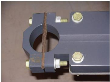
Figure 5 The clamp for the AWI Hydrophone
