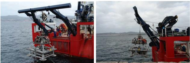
Figure 15 Test of deployment procedure in the harbour of Vigo
