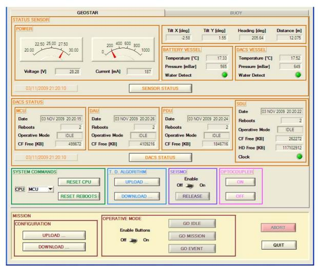
Figure 21 WET test: GEOSTAR status and sensor status request results, obtained with the acoustic link
