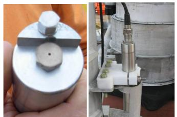
Figure 7 The Paroscientific absolute pressure sensor: the zinc anode and the anti fouling port (left) and the new plastic bearing (right)
