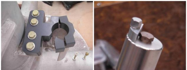
Figure 4 The pressure sensor plastic clamp broken during the assembling (left) and the anticorrosive anode touching the anti-fouling port (right)
