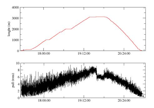
Figure 29 The winch payout (red line) and pull (black line) during the deployment of GEOSTAR
