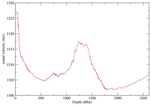
Figure 23 Sound velocity profile from CTD cast in the deployment area
