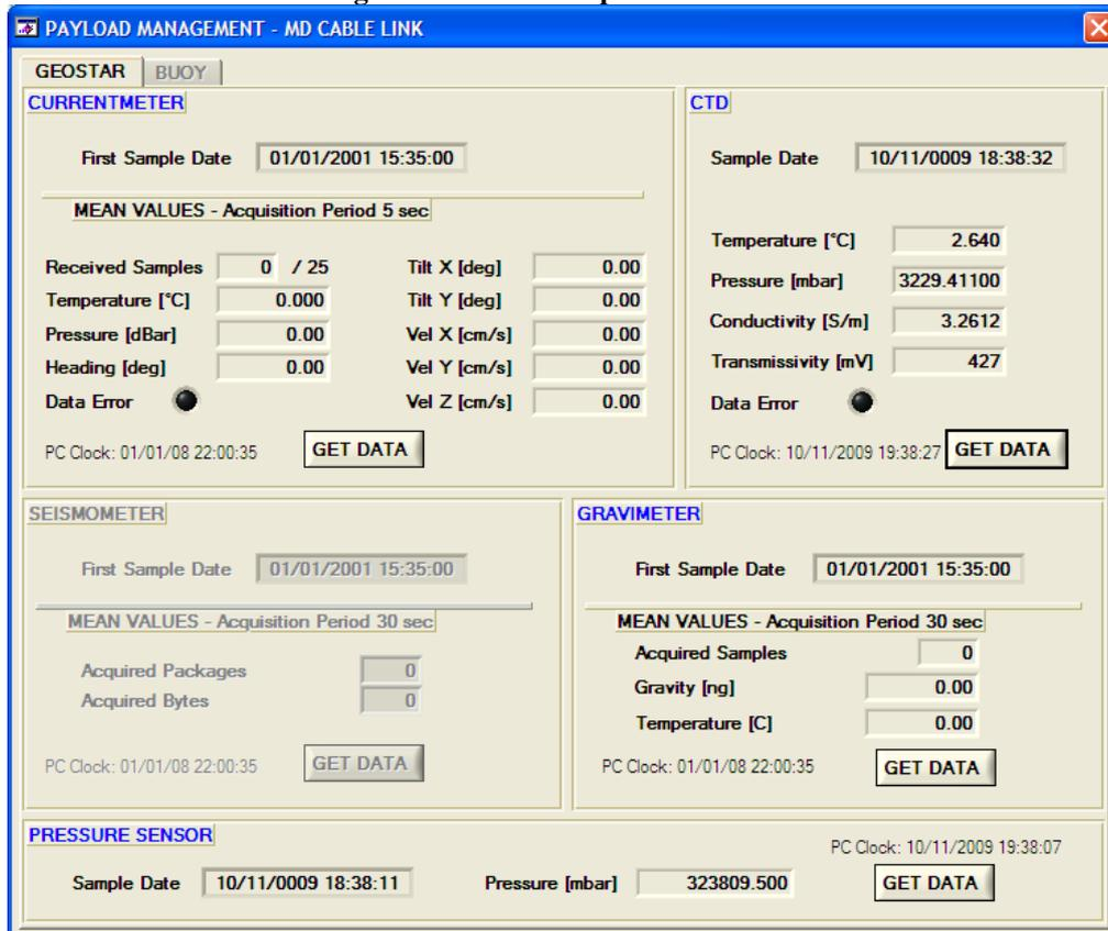
Figure 36 GEOSTAR interrogation after the touch down (pressure and CTD data)
