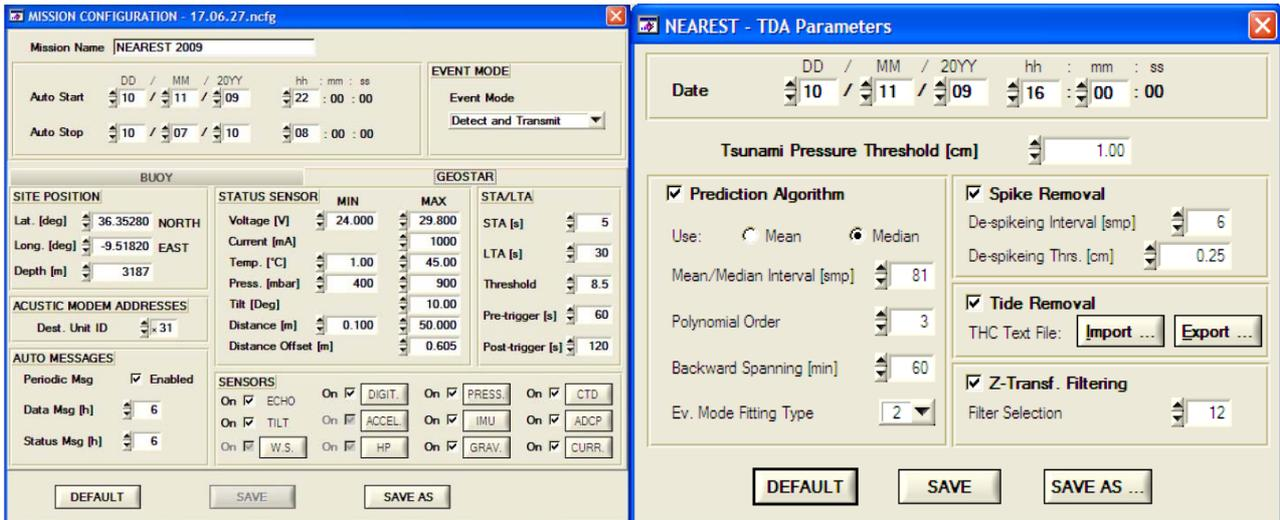
**Figure 28** The mission configuration (left) and the Tsunami Detection Algorithm parameters for the GEOSTAR mission
