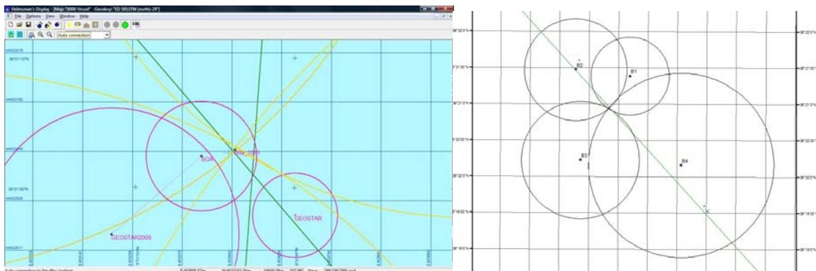
**Figure 25 Geometric determination of dead weight position using 4 point of range measurements. The diagonal green line represent the route followed by the vessel during buoy deployment; The yellow circles are centered each one in the four point of measure; B1-B5 are the points for acoustic localization, the circle intersections localizes the DW position.**
