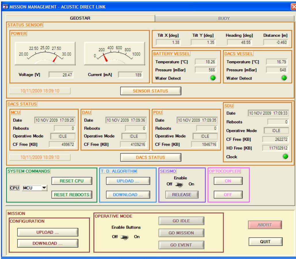
Figure 34 interrogation with acoustic link with GEOSTAR at 1000 m depth
