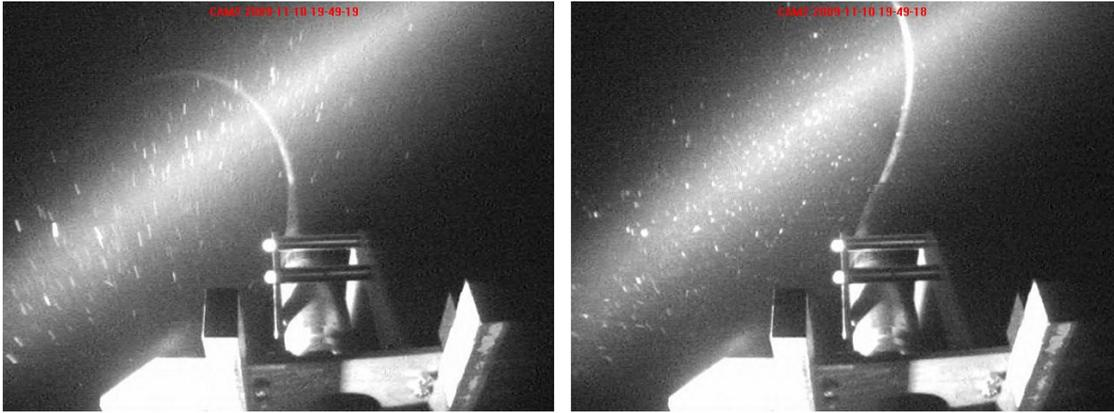
Figure 18 Intense cable-slack events during deployment
