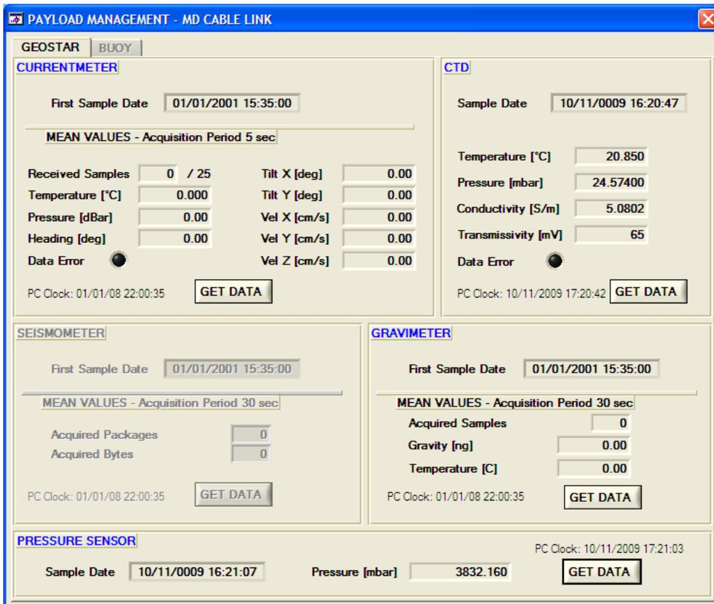
Figure 31 GEOSTAR interrogation (CTD and pressure) just after the station enter the sea water
