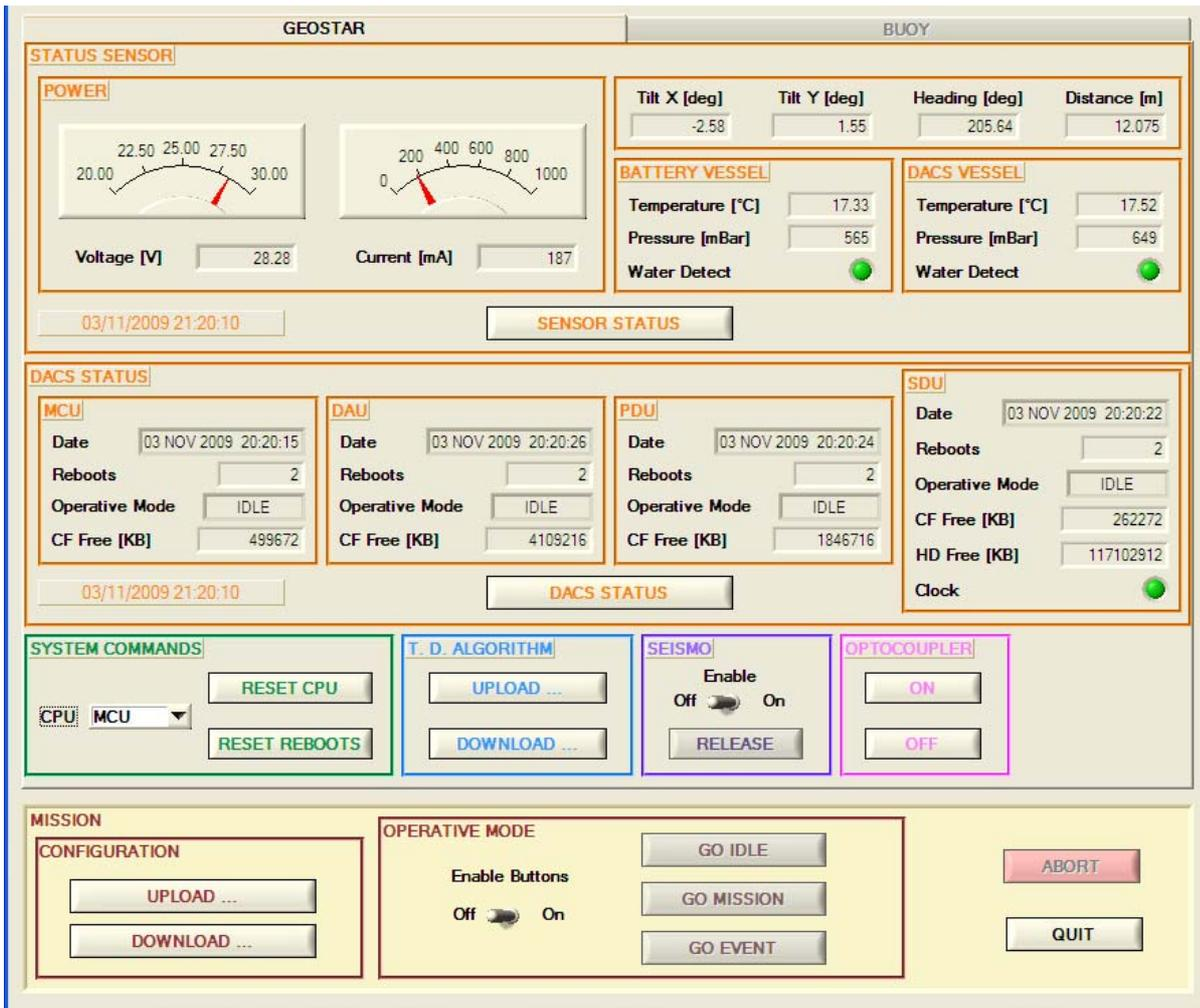
Figure 21 WET test: GEOSTAR status and sensor status request results, obtained with the acoustic link
