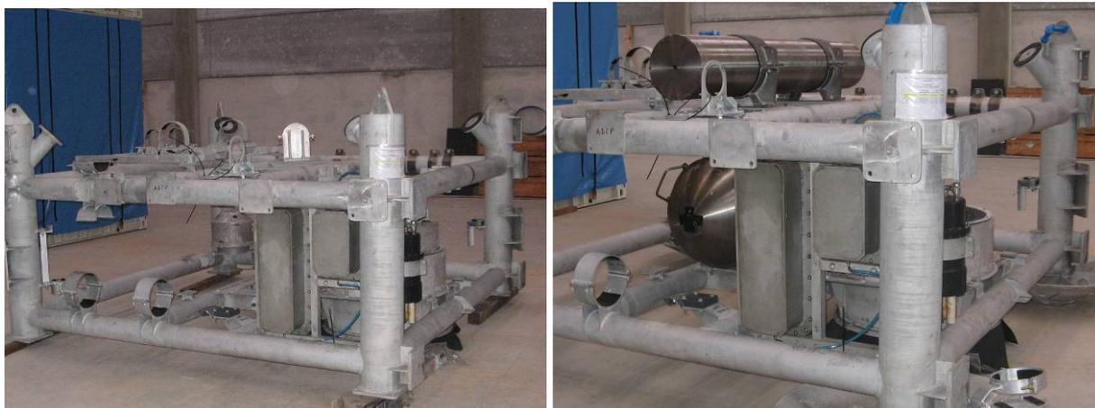
Figure 3 The beginning of the GEOSTAR assembling: the bare frame (left) and with the DACS, the battery vessel and assembled (right) .
