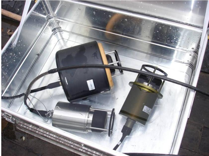
**Figure 11** Acoustic transducer wet test
