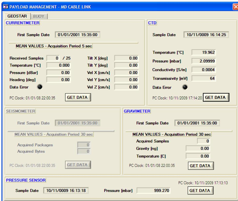
Figure 30 GEOSTAR interrogation (CTD and pressure) just before the deployment (station on the ship deck)
