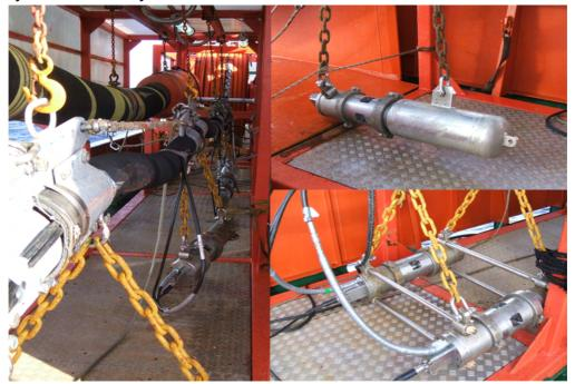
**Figure Al.4.** – Details of airguns, airgun array and cluster used during the survey.
