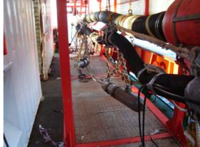
**Figure 29.-** 1000 c.i. airgun, model Bolt 1500LL used in this experiment (left). Detail of the main airgun array (right).
