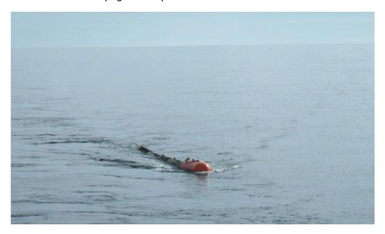
**Figure Al.5.-** Airgun array in the water.
