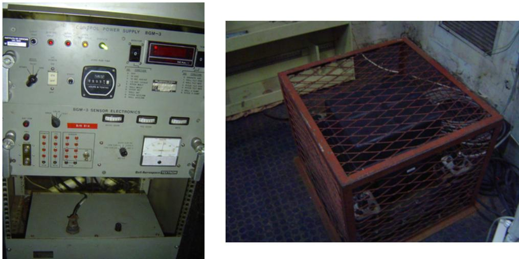
**Figure 23.-** Sensor subsystem front panel (left) and stabilized platform box (right).
