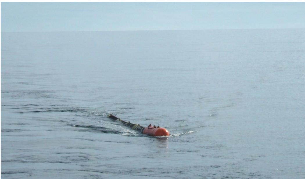
**Figure AI.5.-** Airgun array in the water.
