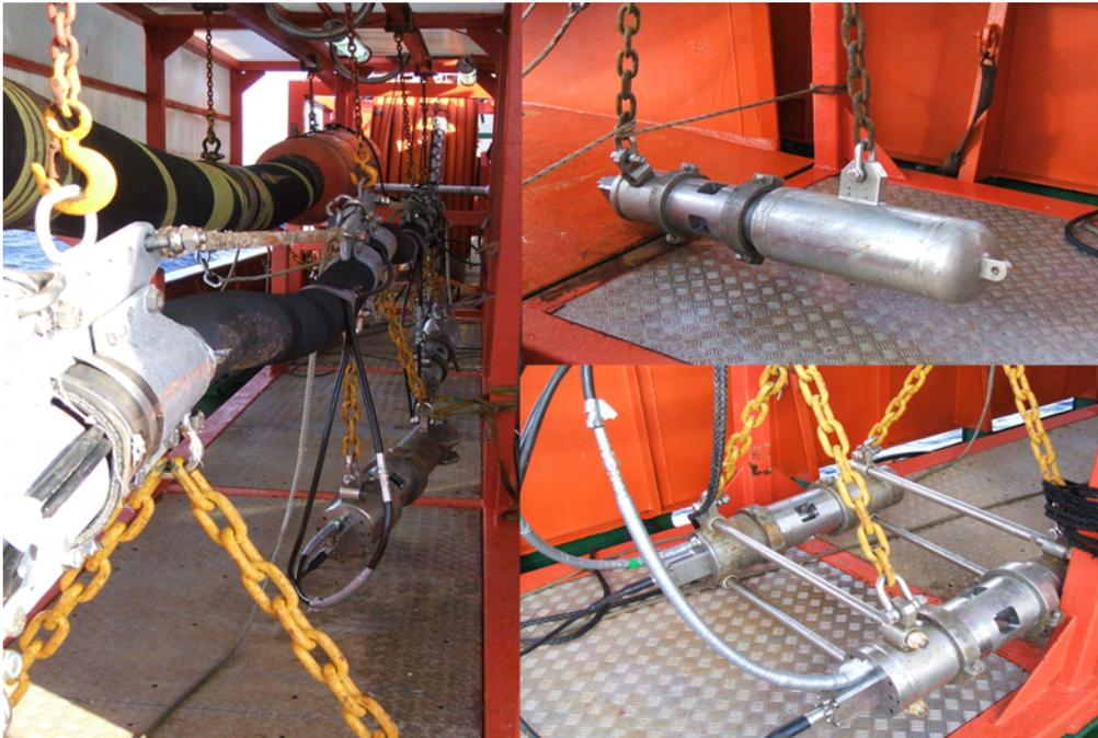
**Figure AI.4.** – Details of airguns, airgun array and cluster used during the survey.
