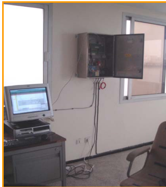
Figure 3.2.4 - Tide gauge configuration, PC data transfer running LogoSens operating program.
