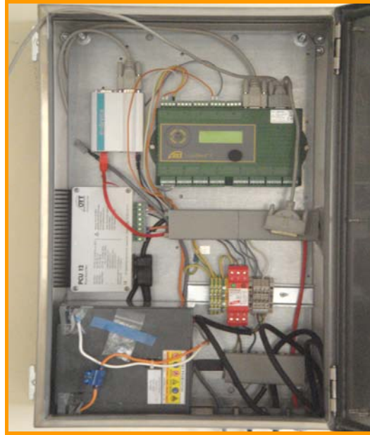
Figure 3.2.3 –Rack containing digital tide gauge modules
