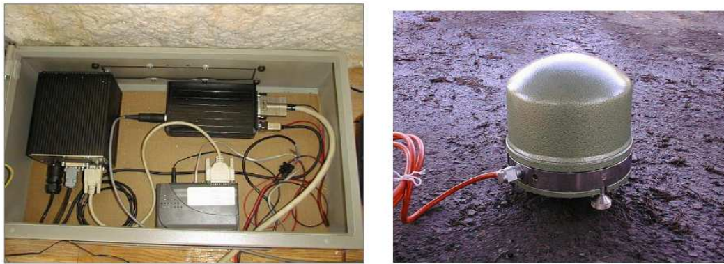
Figure 10. Field elements that conforms the broad band seismic station. Left: Earth Data 24 bits PS2400 digitizer, modem and Pc interface where the data are locally stored in at 30 Gbytes hard disk. Right: triaxial Streckeisen STS-2 broad band seismometer.
