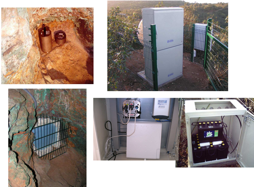
Figure 2. Seismic station of Vaqueiros (PVAQ), Algarve (Installed on an old mine). Left: Guralp 3T broadband seismometer and Guralp 5T accelerometer; Earth Data 24 bits PS2400 digitizer, modem and Pc interface where the data are locally stored in at 30 Gbytes hard disk. Right: Seiscomp PC (storage disk for 60 days of autonomy), VSAT modem unit, batteries (communications autonomy for 4 days; data acquisition autonomy of 10 days), charging control unit).
